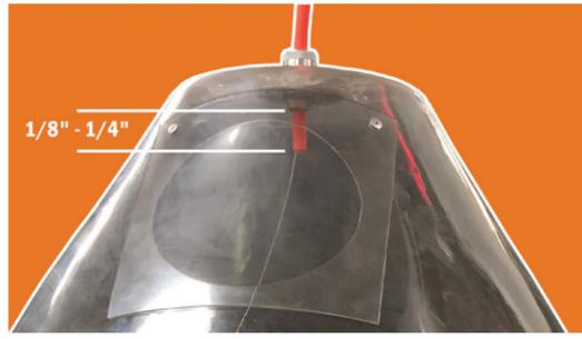
Remove any burrs or flashing at both ends of the Drum Tube (C) and connect to the Drum Tube Connect Kit of Step 1, allowing the Tube to protrude 1/8" - 1/4" below the Connect Kit.
