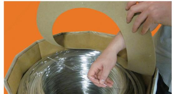
Grasp the end of the wire while removing and discarding the cardboard ring. Pressure should be applied to the wire to prevent it from springing out of the drum.
