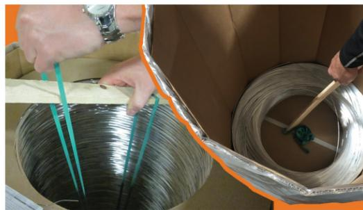
Remove the wood slats and release the rubber bands. Center the rubber bands in the bottom of the drum so they are not touching the wire. **Failure to do so may lead to wire tangles.**
