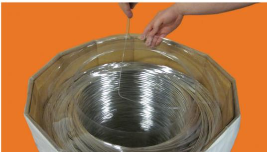
Thread the wire through the inside of the plastic float ring (E) and then rest the float ring on the wire. The apex of the float ring's curvature should point DOWN.
