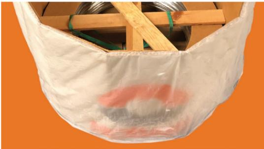
Remove the lid from the drum. Remove the wire tie on the plastic bag and then pull the bag down over the drum.
