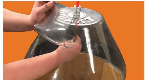
Thread wire into the drum tube. Push wire through the tube into feed roll system. Jog the wire out of the contact tube several feet. Clip and discard the protruding wire.
