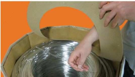
Grasp the end of the wire while removing and discarding the cardboard ring. Pressure should be applied to the wire to prevent it from springing out of the drum.
