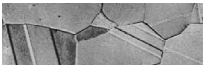
Figure 26 – Photomicrograph of austenite.
