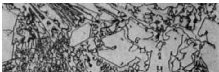
Figure 28 – Photomicrograph Of Large Carbides In A Carbide Eutectic Matrix.
