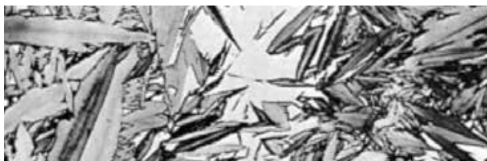
Figure 27 – Photomicrograph Of Martensite.
