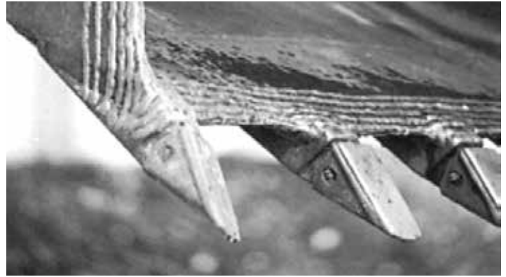
Figure 6 – OVERLAY - bucket lip hardfaced as preventive maintenance
