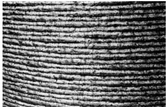
Figure 25 – Stress relief cracks in a high chrome carbide overlay.
