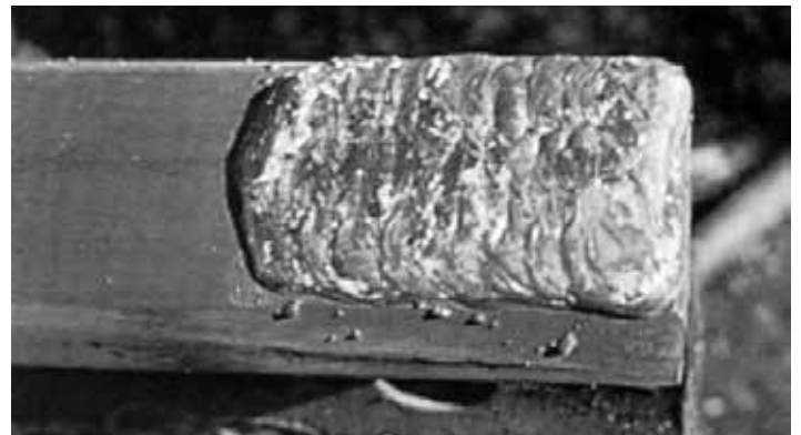
Figure 5 – BUILD-UP - worn rail end rebuilt past original dimensions-it will be ground prior to service
