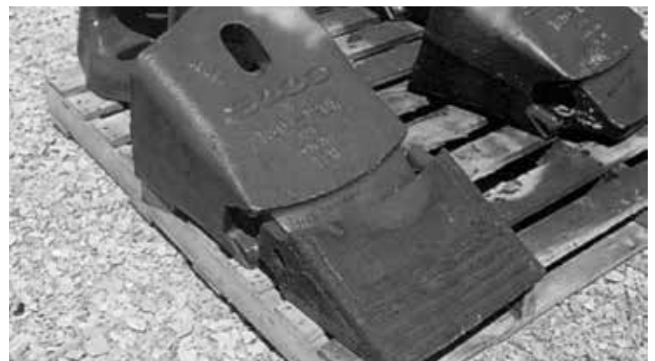
Figure 7 – OVERLAY - replacement dragline bucket tooth hardfaced as new equipment
