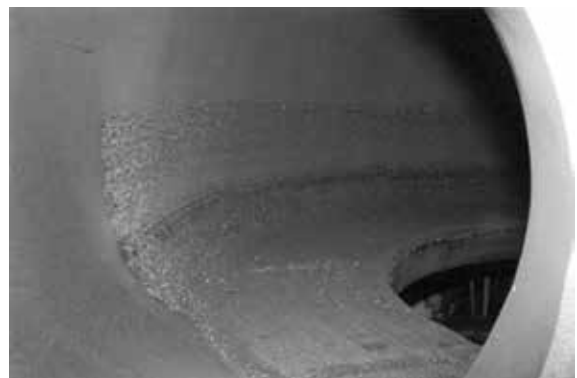
Inside View of Worn and Partially Rebuilt Dredge Pump Shells
