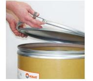
2. Release metal ring that secures the lid to the chime ring. Remove band of tape that seals the lid to the chime ring.
