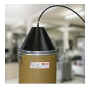
Pull or push the wire through the conduit cable and secure connection with the wire feeder. Setup is complete.
