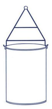
The drum ring shall remain stationary during use. Do not rotate during use. Keep moisture out.
