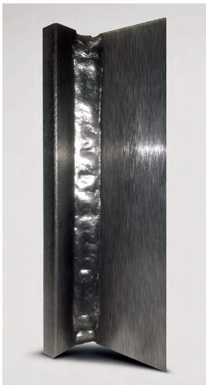
Fig. 3 — In terms of welding operator skill and technique, out-of-position FCAW-G requires less manipulation or weaving to achieve the ideal weld contour (as shown with this weld).
