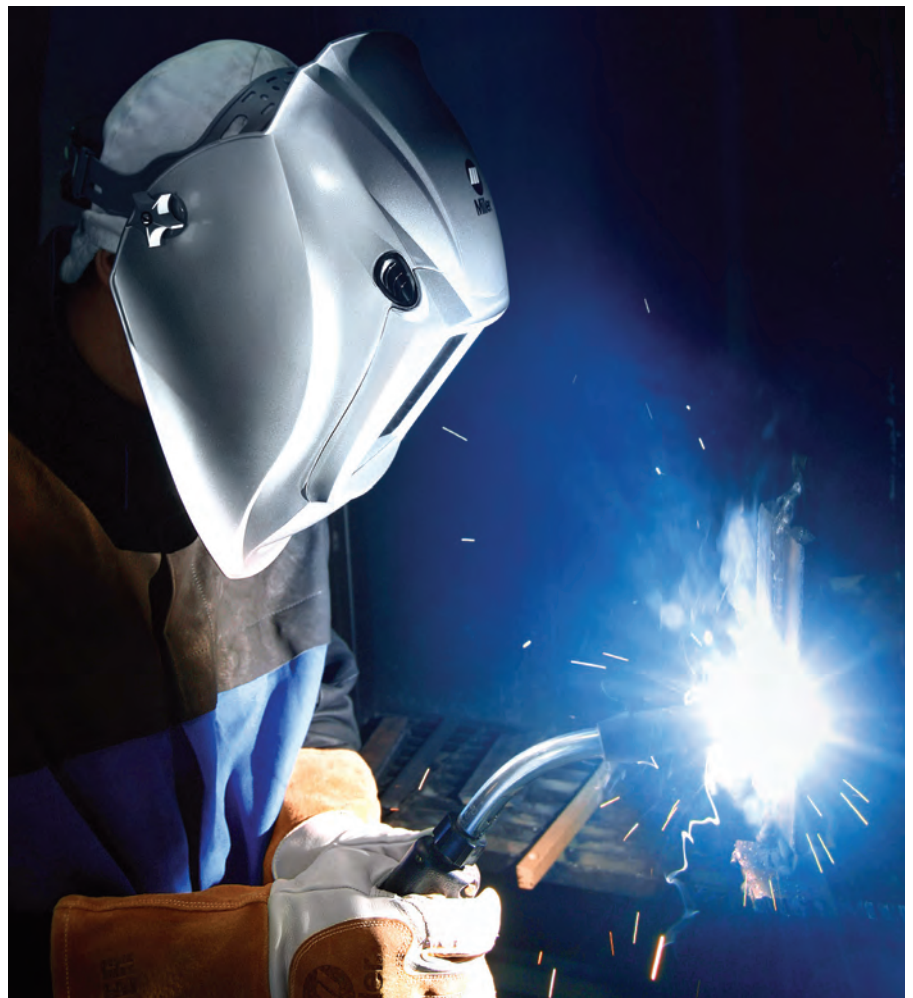
Fig. 1 — Gravity is the biggest challenge when welding out of position because the weld pool drips downward, which makes it harder to produce quality welds and maintain higher levels of productivity.
