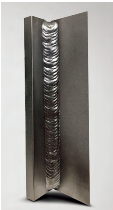
Fig. 2 — For out-of-position GMAW, the welding operator will often be required to employ a weave technique to obtain the acceptable bead shape and fully wet into the toes of the weld.
