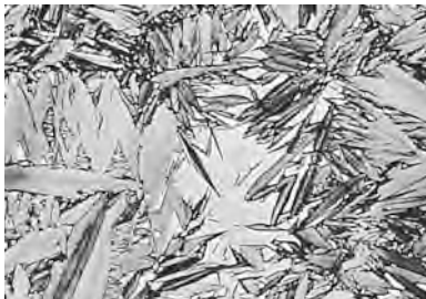
Photomicrograph of martensite.
