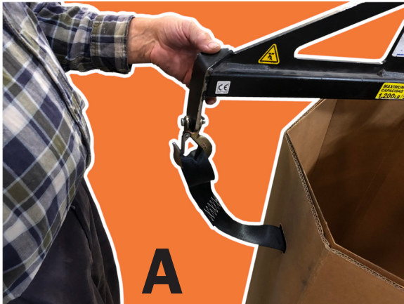
A: Ensure the lifting device has a locking device, and that the strap is clear of the locking device. B: Improper Technique. Ensure the lifting device is centered over the load to prevent the risk of swinging.
