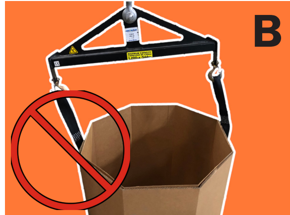
A: Ensure the lifting device has a locking device, and that the strap is clear of the locking device. B: Improper Technique. Ensure the lifting device is centered over the load to prevent the risk of swinging.
