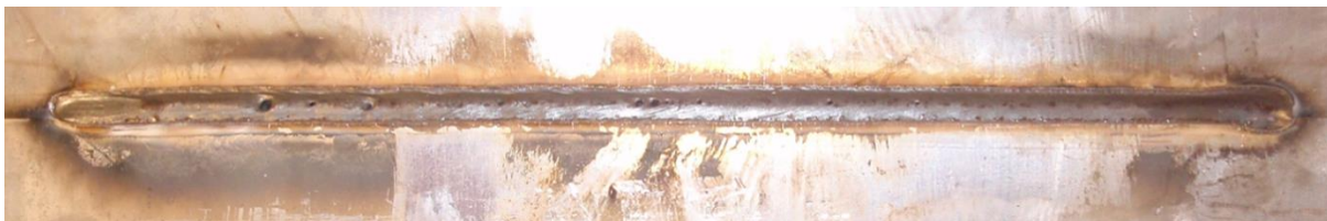
Figure 6. Sample S-2, which was produced using ER70S-6 at 89 cm/min (35 ipm) and contained 0.05% porosity.
