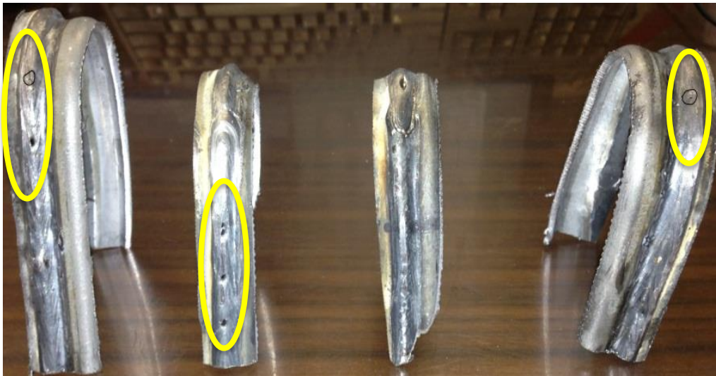
Figure 14. Bend test samples produced at customer location using ER70S-3. Note that porosity that was present in the weld has opened up during bend testing.
