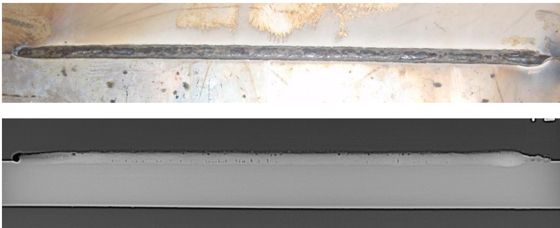
Figure 12. Sample F-12, produced using E71T-14 (1.92% porosity).
