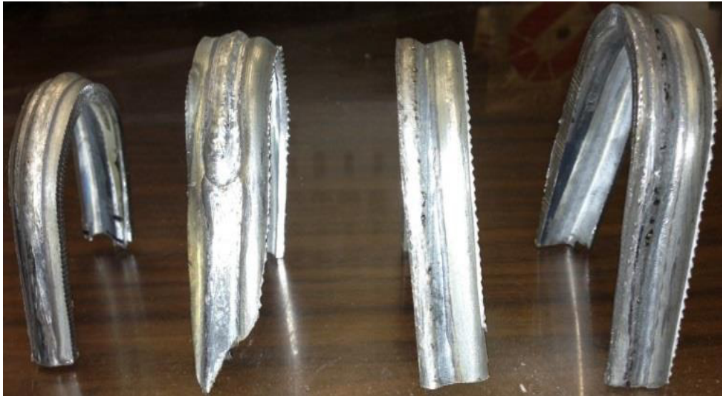
Figure 15. Bend test samples produced at customer location using FabCOR F6. Note that there is no evidence of porosity.
