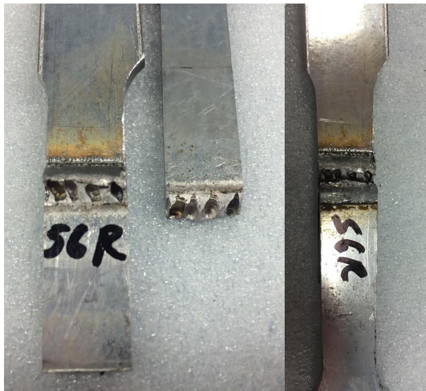
Figure 8. Typical tensile failure in sample containing porosity. Example shown is Sample S6 [ER70S-6, 64 cm/sec (25 ipm), 7.27% overall porosity].
