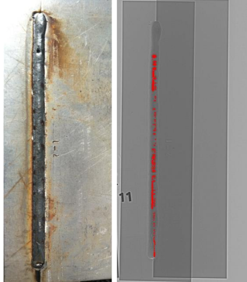
Figure 1. Example of weld produced with solid wire GMAW that passed visual inspection. The weld had gross internal piping porosity, as indicated in red.
